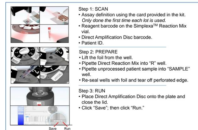
Figure 1. Simplexa Direct Assay Setup
